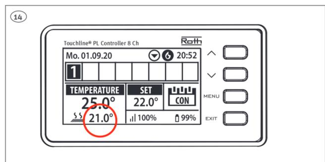
**(UK)** In the overview you can see both the thermostat (setpoint 22,0°C, actual 25,0°C) and the actual floor temperature (21,0°C). Repeat this for all other zones/channels (2 to 8) with a floor sensor.
